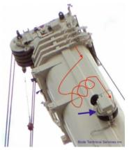
STEP 2 – With the drum clamped to avoid turning, slide the loose length cable carefully behind the drum and re-loop it by hand back onto the drum. Keep in mind you are not turning the drum, just laying cable on by hand.
