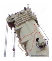
STEP 1 – With a fully retracted boom, pull 1 – 5 wraps of length cable off the drum by carefully turning the drum counter-clockwise. Clamp the drum side plates with vice grips to hold it securely and prevent any rotation.
