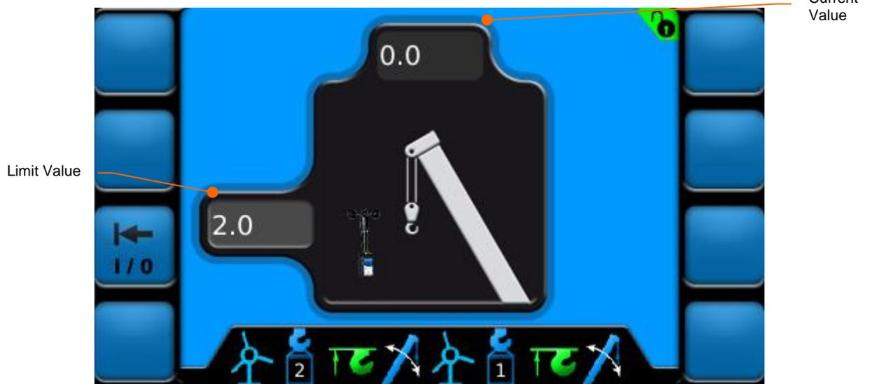
**Figure 9: Set Wind Sensor Limit Screen**
