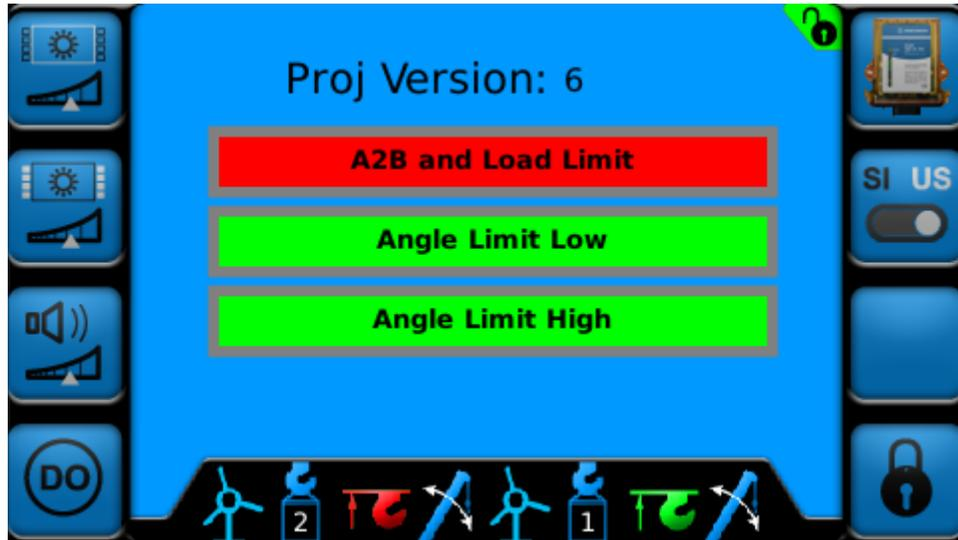
Figure 16: Digital Output Screen with DO1 Low
