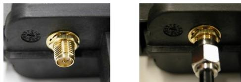
Figure 21: Connecting Antenna to TRS10-W2
