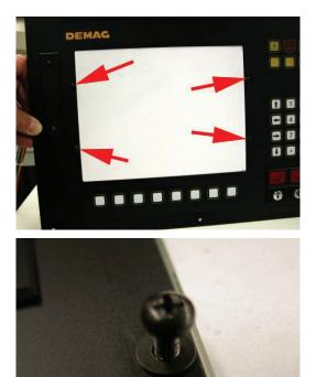
• Set the plexiglass plate in place on the back (with the milling groove on the left) and ...
