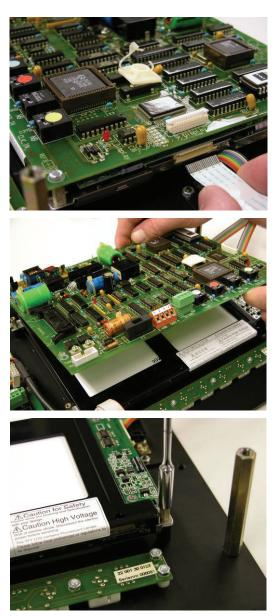
• Loosen the other side of the ribbon cable as well. Then remove the locking frame.
