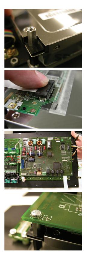
• ...and fasten with four spacing bolts (3).
