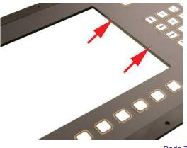
• Drill out the four threadings that are present with a drill and 3.5-mm bit.
