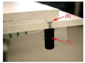
• Prepare the plexiglass plate from the conversion kit with counter sunk screw (6) and spacing bolts, black (7) as shown.
