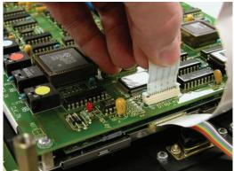
• Remove the remaining plug connections.
