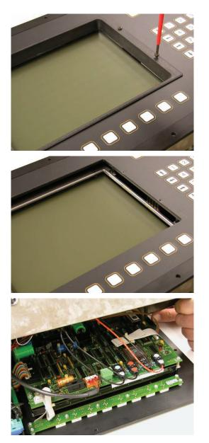
• Using a Phillips screwdriver, unscrew the 4 screws on the tube.
